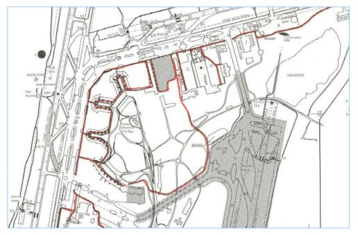
The road system (marked in red) for the terminals and ramps at Arlanda airport
