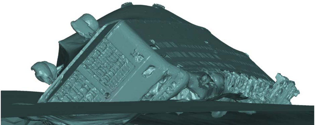
Figure 45. Outward deformation at the port side of Deck 7.
