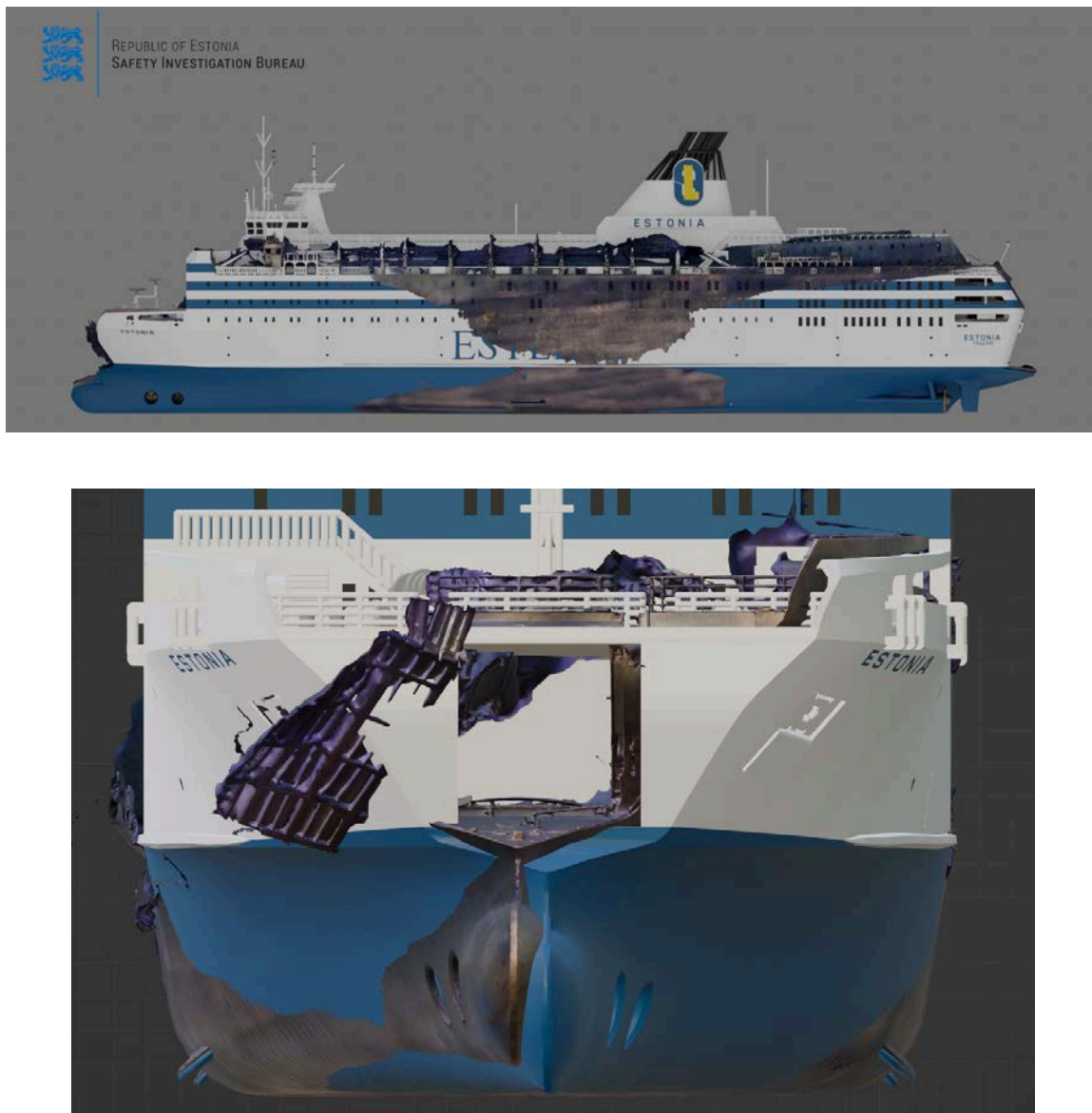
Figure 42. Hull deflection at the port side ( above ) and at the bow ( below ). (Overlay of the intact ship with the photogrammetric model of the shipwreck in provided by Estonian Safety Investigation Bureau)
